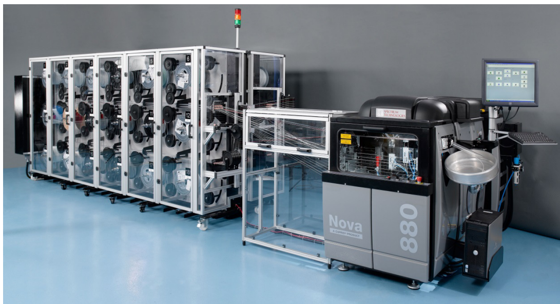
Figure 2. Automated Nova 880 with 32 station dereeler and 32 station ASL wire Auto Select & Load facility.
